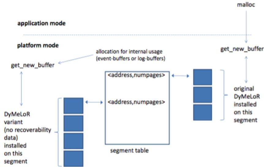
Figure 4.6: Memory Allocation for Platform and Application Usage
