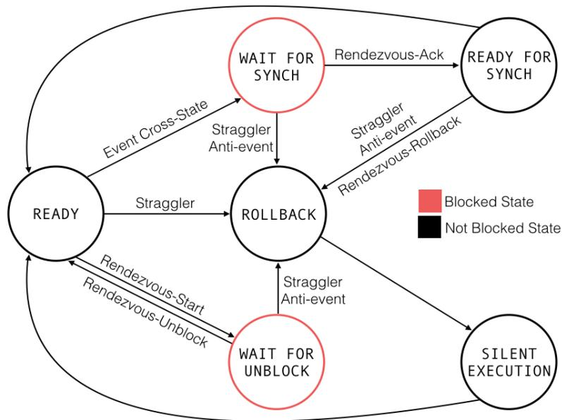
Figure 5.12: State diagram of simulation object
