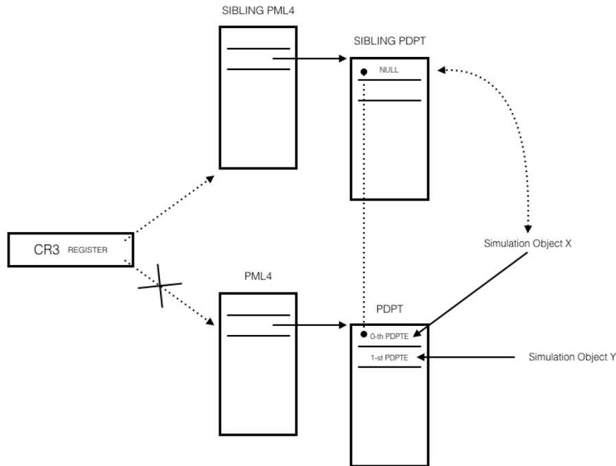
Figure 5.4: Memory Stock of  $LP_x$  is opened to the current Worker Thread
