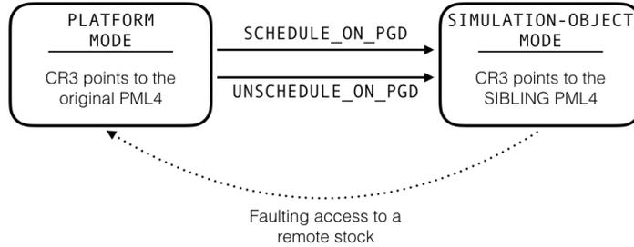
Figure 5.5: State diagram of simulation object according to the value of CR3
