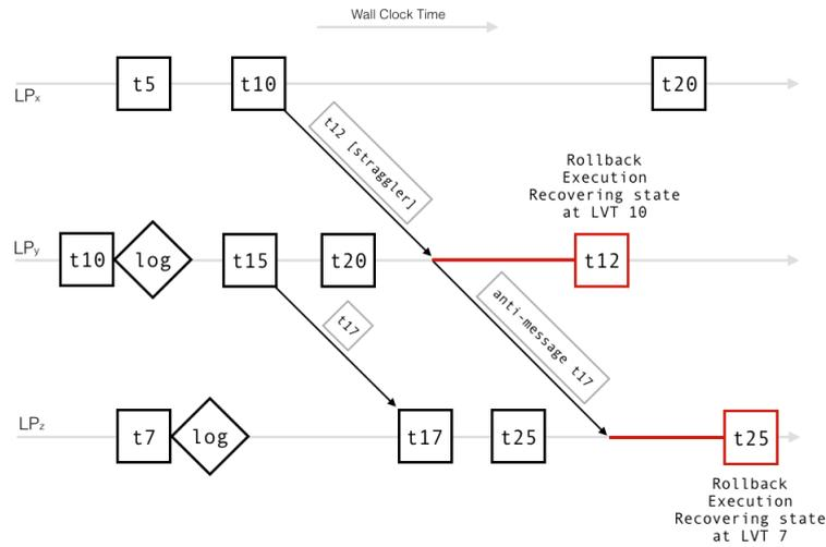
Figure 2.3: Rollback work flow
