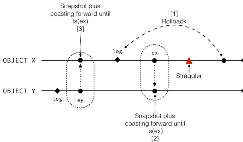
Figure 5.8: Example where rendezvous events generate cascading rollbacks
