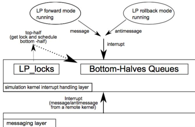
Figure 4.1: Top/bottom Halves Architecture
