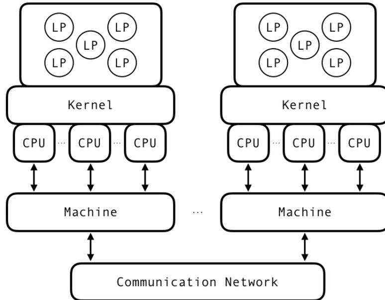
Figure 2.1: System Architecture: Symmetric Multi-Threaded Simulation Kernel
