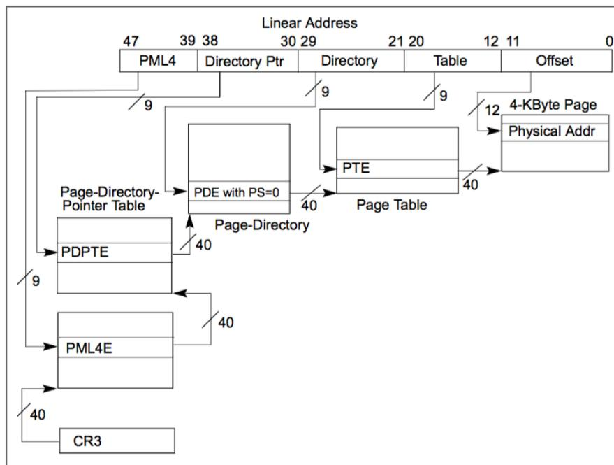
Figure 5.2: Linear-address translation to a 4-KByte page using IA-32e Paging
