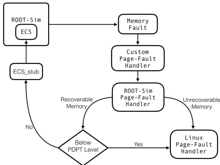
Figure 5.11: Execution flow of ESC tracking
