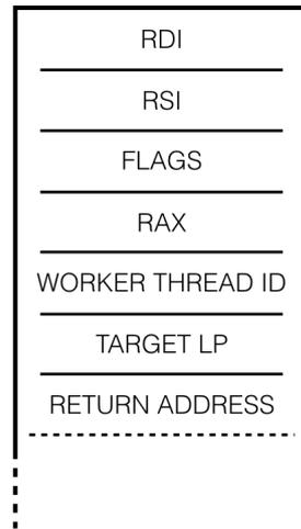
Figure 5.10: How ROOT-Sim page-fault handler left the stack
