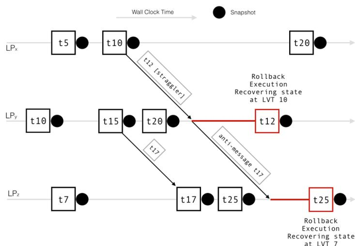
Figure 2.4: Example of rollback in case of CSS
